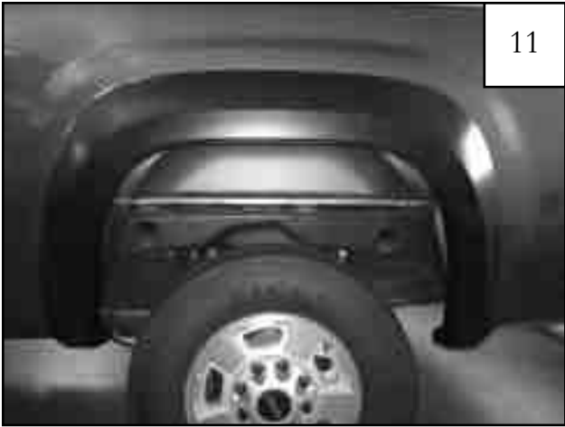
Completed rear flare installation.
