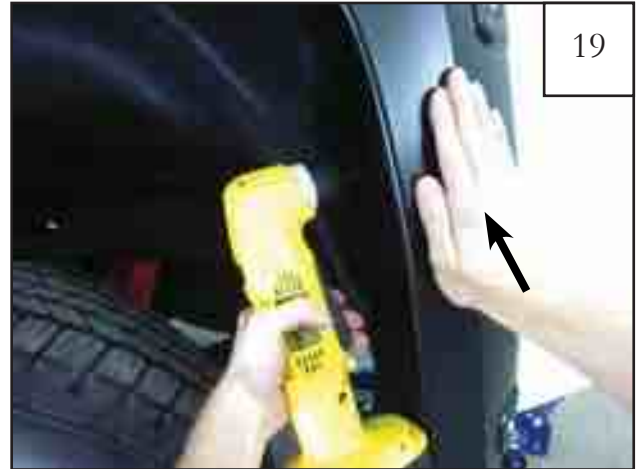
Install self-tapping screws (SW1-0066) into pilot holes drilled in step 17 (3 places). Press flare firmly towards the vehicle while fully tightening.
