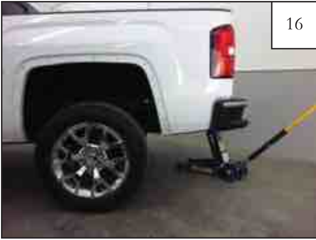
Rear fender/truck bed must be raised to gain access for drilling. Use a floor jack on the rear hitch to raise the truck bed, or remove the rear tire to allow clearance for drilling.
