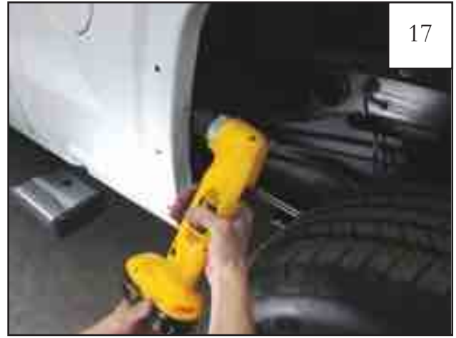
Using a 3/32" drill bit, drill pilot holes through sheet metal at the marks made in Step 15.
