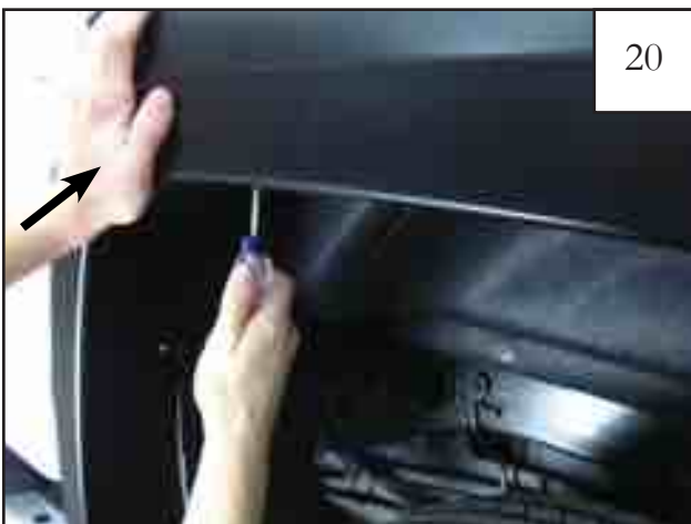
Press flare towards vehicle and fully tighten all remaining fasteners.
