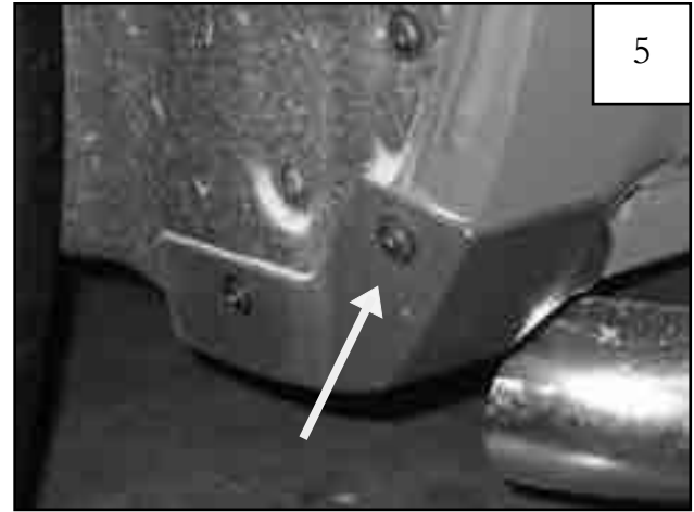
Using a T-15 Torx bit, remove two factory screws in mudguard at rear of front wheel well.
