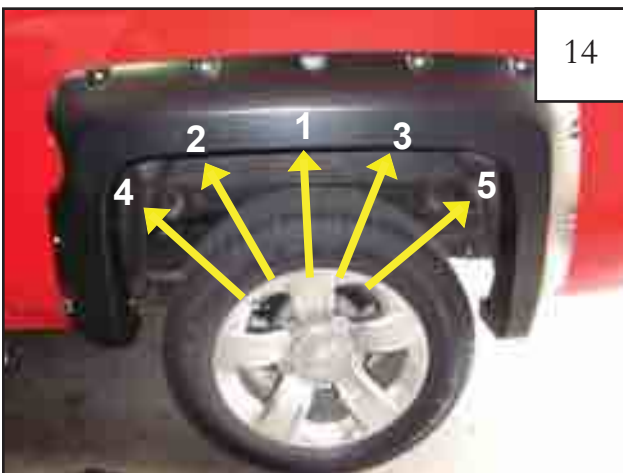
Install supplied self-tapping screws (SW1-0066) into pilot holes in the order indicated. TIGHTEN ALL SCREWS
