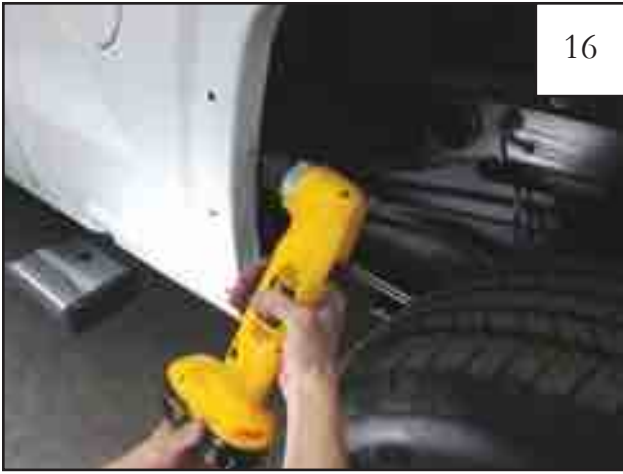
Using a 3/32" drill bit, drill pilot holes through sheet metal at the marks made in Step 34.
