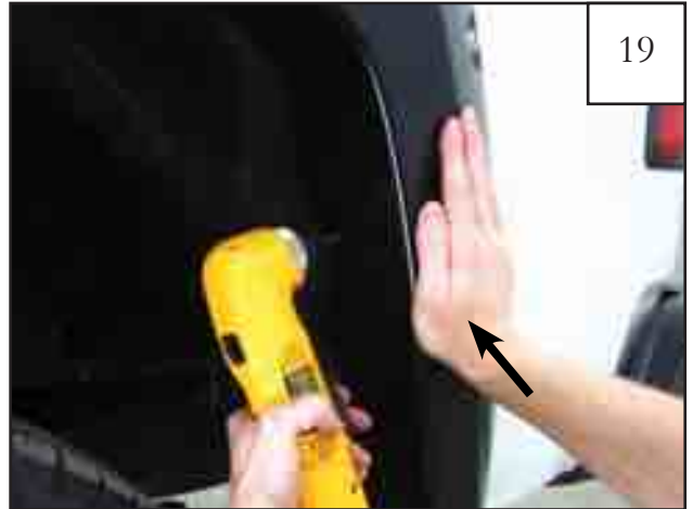
Install self-tapping screws (SW1-0015) into pilot holes drilled in step 36 (3 places). Press flare firmly towards the vehicle while fully tightening.
