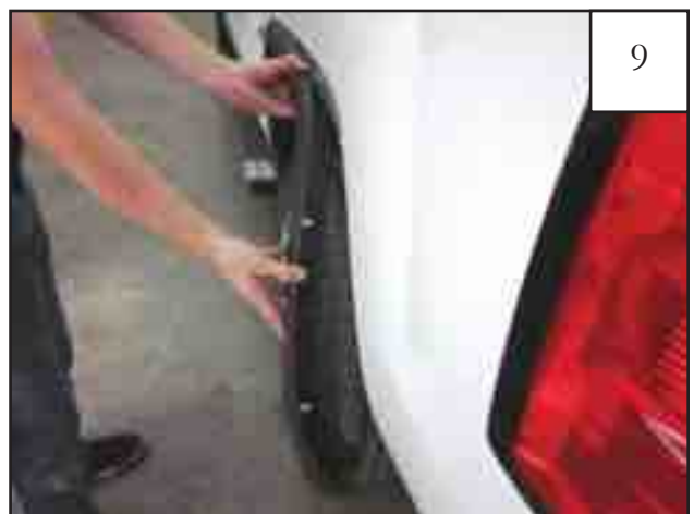
Starting at the lower rear end of the factory flare, firmly grip part and pull to remove from vehicle. Note: You will hear popping sounds as the factory fasteners release from vehicle. This is normal.
