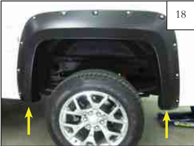
Reinstall the lower 2 factory fasteners removed in step 27 using a 10mm deep socket and wrench.
