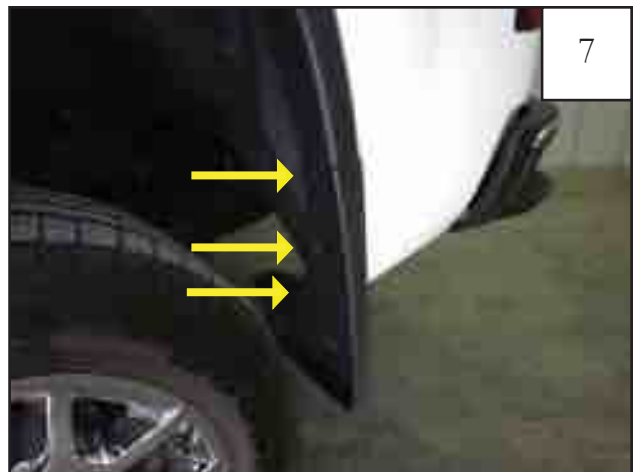
FOR MODELS WITH FACTORY MUDFLAP: Use a Phillips Head Screwdriver to remove 3 factory mud flap fasteners.
