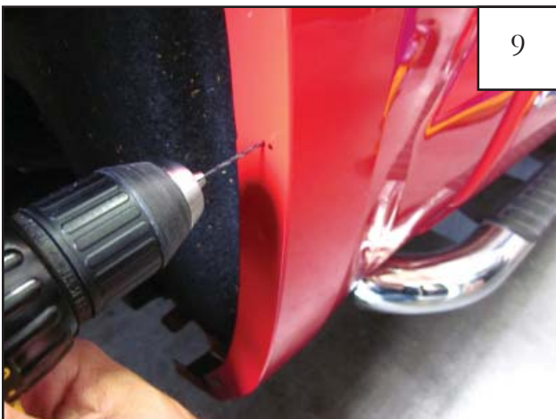
Using a 3/32" drill bit, drill pilot holes at the marks made in Step 8.
