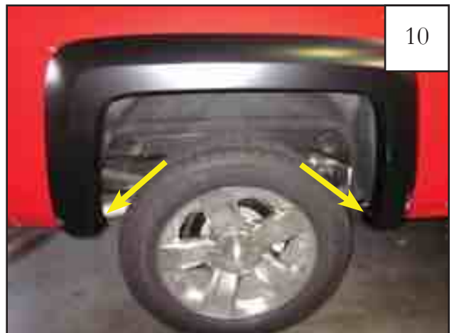
Re-install supplied screws (SW1-0056) into two lower most holes.
