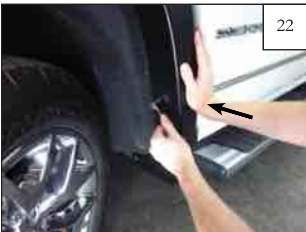
FOR MODELS WITH FACTORY MUDFLAP: Reinstall factory fastener removed from mudflap in step 5. Press flare towards vehicle while fully tightening using a T-30 Torx Bit.
