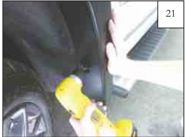
Install self-tapping screw (SW1-0066) into pilot hole drilled in step 16. Press flare towards vehicle while fully tightening. Note: This step not needed for models with factory installed mudflaps.
