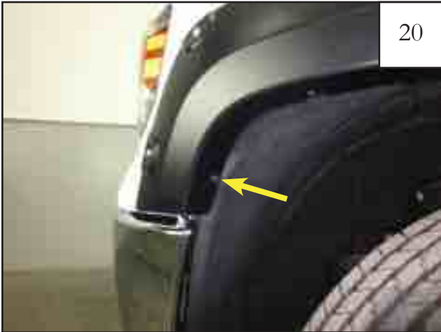
While holding Flare on vehicle, install factory screw removed in step 7 through flare and into factory hole. Do not fully tighten at this time.
