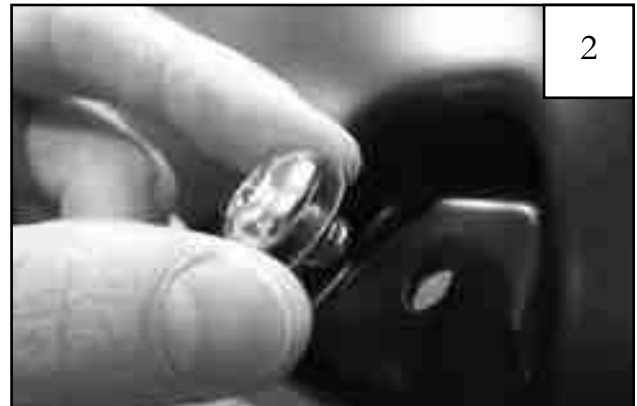
Put each Bolt/Washer combination through a pocket hole in the flare, Bolt head and Washer on the outside.
