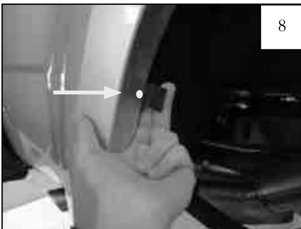
Wrap five supplied tabs (MT1-0034) around inner lip of sheet metal over the marked locations.
