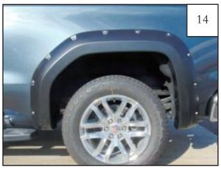
Fully tighten all fasteners, then replace the rear wheel as instructed in your user's manual.
