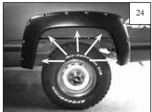
Applying moderate pressure to outside surface of flare, tighten all screws beginning with the two corner locations and then the remaining screws.
