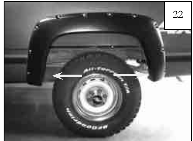
Reposition flare on fender. Start supplied Screw (SW1-0050) through two corner hole locations and through each Clip (CL1-0005) installed in step 20. If needed, use awl to align holes with the installed clips.
