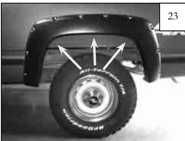
Ensuring flare is properly located on fender, start supplied screws (SW1-0050) through each of the remaining holes.
