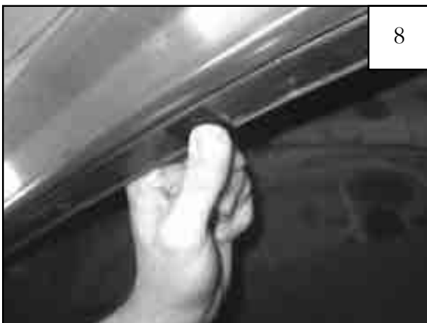
Remove flare. Center a supplied Tab (MT1-0002) over the marks made in step 6, aligning edge of tab with inside edge of fender lip (tab may extend over outside of fender).
