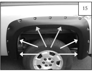
Fully tighten all screws starting with the newly installed Screws (SW1-0058) in upper two hole locations while pressing in on flare to ensure it is snug against sheet metal.
