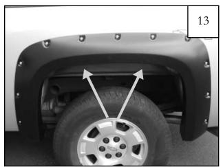
Reposition flare on fender. Start a supplied Screw (SW1-0058) through upper two hole locations and through each Clip (CL1-0022) installed in step 11. If needed, use awl to locate holes thru tabs installed in step 10.
