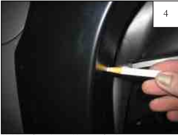
4 Holding flare in position on fender, use a grease pencil to mark six hole locations.
