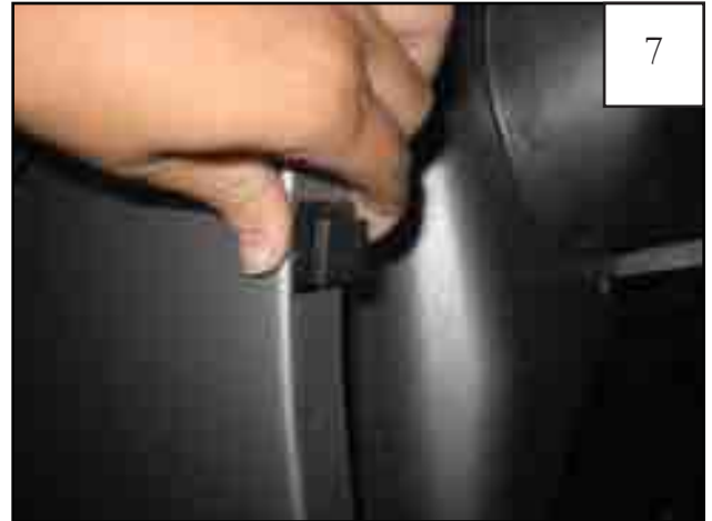
7 Slide a supplied clip over each black tab. Clips may need to be adjusted to align with holes in flare.
