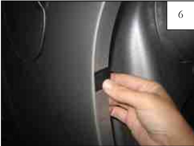
6 Center a supplied black plastic tab over each mark made in Step 3, aligning edge of tab with inside of fender lip (tab may extend over outside of fender).
