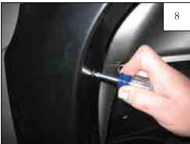
8 Reposition flare on fender. Start a supplied serrated-flange screw through the hole in the flare, and into each clip.
