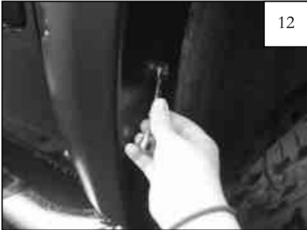
Holding flare in position on fender, reinstall six screws as shown in Step 18.
