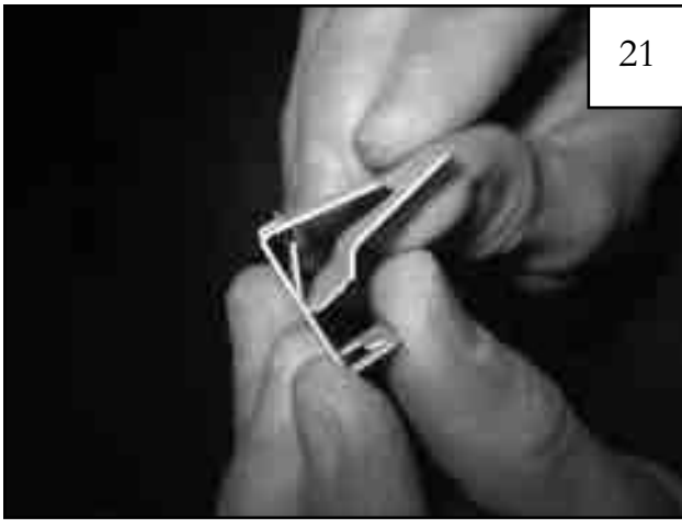
Slide Clip (CL1-0008) into Clip (CL1-0010) as shown. Do not snap clips shut.
