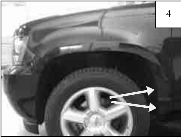
Using a 7mm socket, remove two factory screws. Retain screws for later use.
