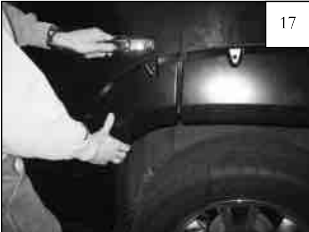
Position Door Piece correctly on door using Rear Flare as a guide.
