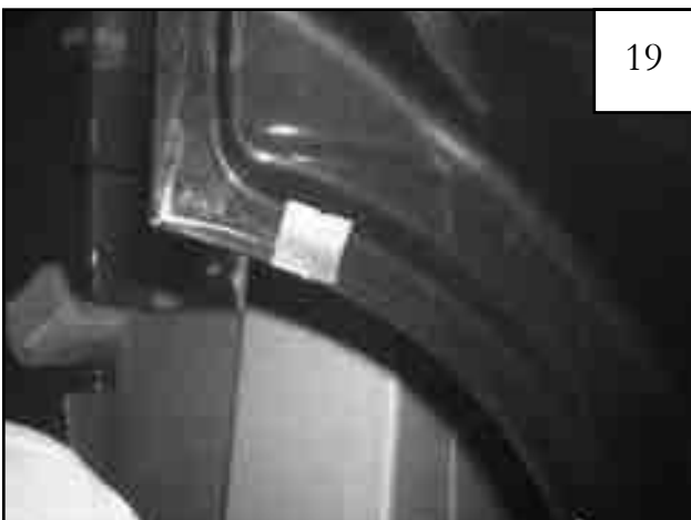
Apply a supplied Tab (MT1-0001) to the inside of the door, centering tabs over the marks made in Step 18 (4 places).
