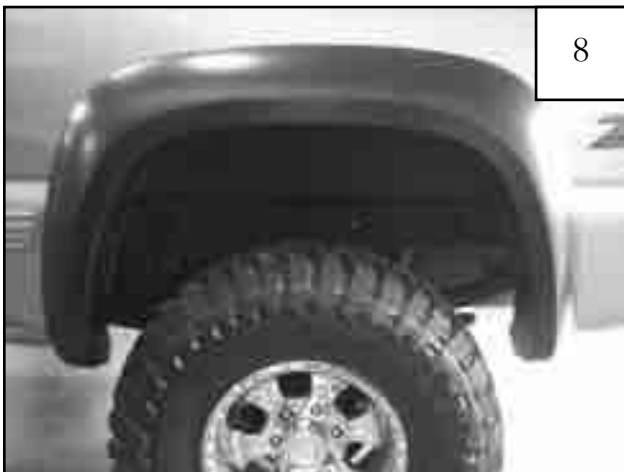
Completed rear flare installation.
