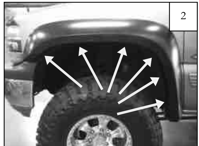
Install six tuflocks using a #2 stubby screwdriver.
