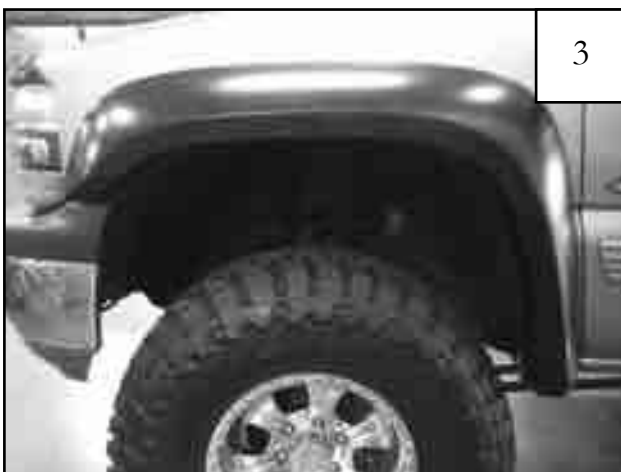
Completed front flare installation.
