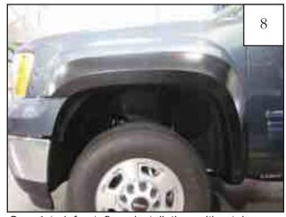
Completed front flare installation without bumper piece.
