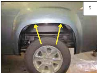
Remove factory mudflap if applicable. Remove and discard two factory installed plastic retainers in top (outer) hole locations of sheet metal (ignore center location). NOTE: If fender liner is installed, remove factory tuflocs.
