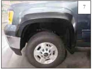
**OPTIONAL BUMPER PIECE:** Completed front flare installation.
