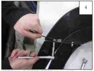
**OPTIONAL BUMPER PIECE:** Using 3/8" and 7/16" wrenches, attach bumper piece to flare using supplied Screw (SW1-0005) and Nut (NU1-0015). Make sure both pieces are properly aligned before tightening. *NOTE: Do not overtighten or parts will warp.*
