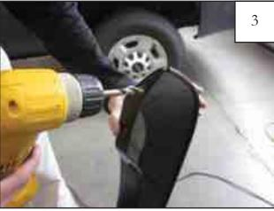
**OPTIONAL BUMPER PIECE:** Using a 5/16" drill bit, drill two holes in dimpled hole locations for both flare and bumper piece. Note: Holes only need to be drilled if bumper piece is being used.
