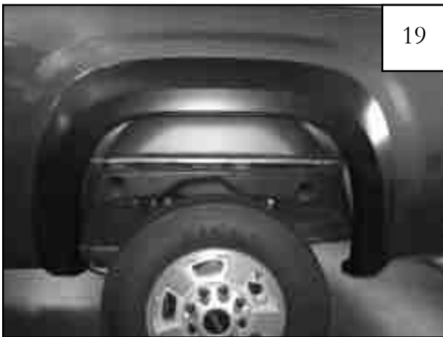
Completed rear flare installation.
