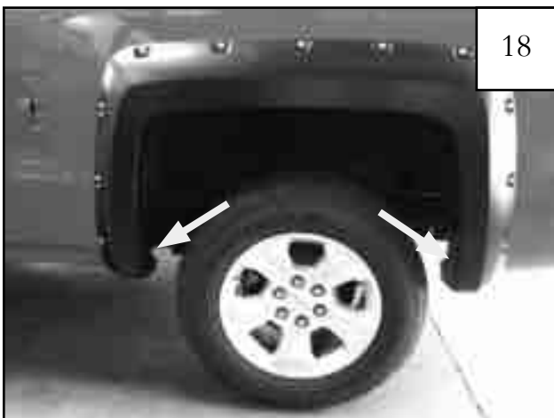
Hold flare firmly in place on fender. Start supplied screw (SW1-0056) at bottom most screw locations (shown). Do not tighten.
