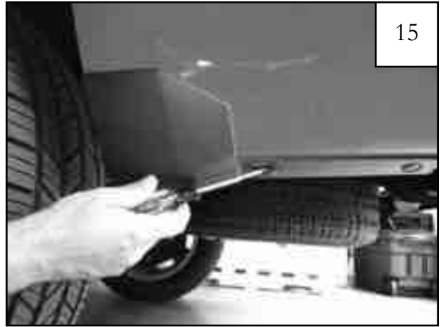
Using a pry tool, remove factory retainers in bottom of factory mudguard. Remove mudguard and discard.
