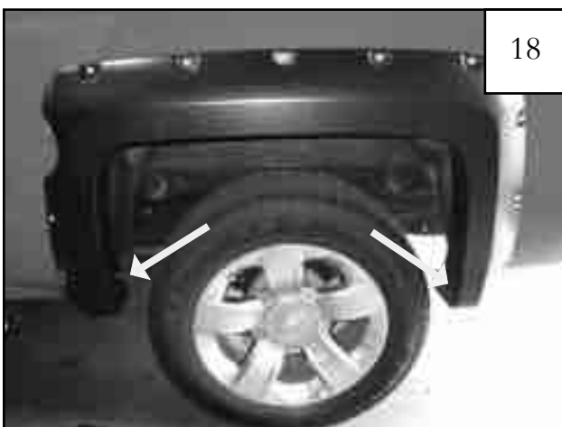
Hold flare firmly in place on fender. Start supplied screw (SW1-0056) at bottom most screw locations (shown). Do not tighten.
