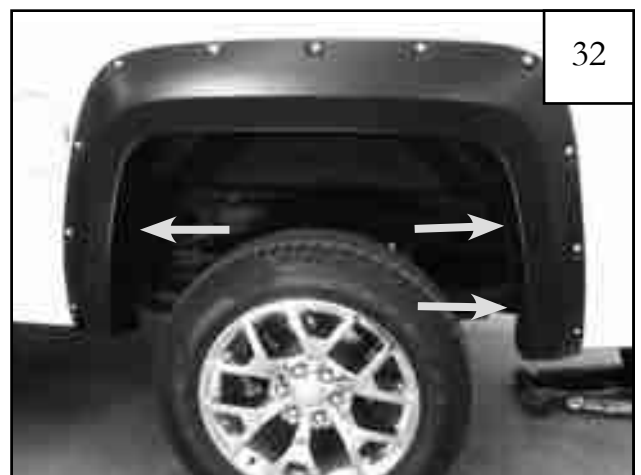
Hole locations to be marked for drilling.
