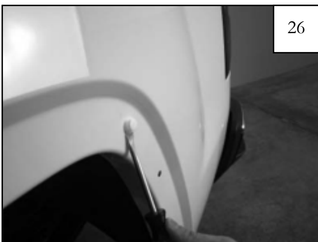
Use a pry tool to remove any remaining factory fasteners that may have stayed on the vehicle during the removal process.
