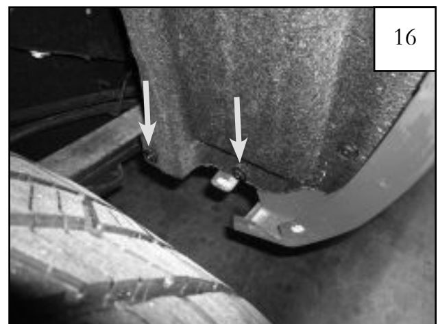
16 Re-install two factory screws into wheel well liner.
