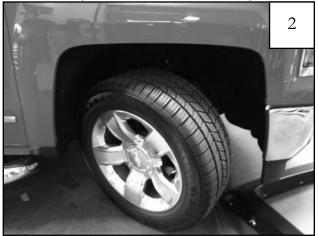
Turn front tire outward for easier installation.
