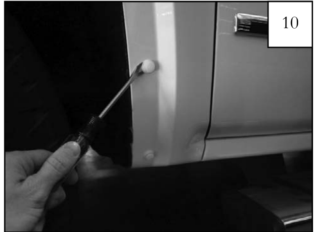
Use a pry tool to remove any remaining factory fasteners that may have stayed on the vehicle during the removal process.
