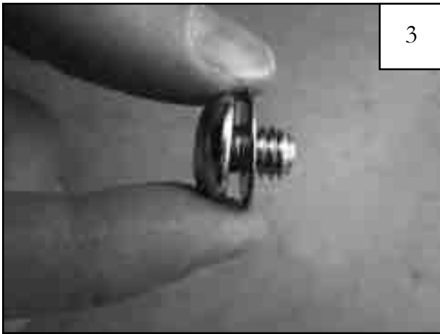
Put a Washer (WA1-0012) on each Bolt (SW1-0067).
