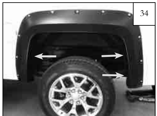
Hole locations to be marked for drilling.
