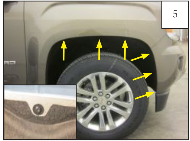
Using a T-15 torx bit, remove six factory fasteners from wheel well. Retain for bracket installation.
