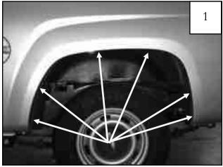
There are six factory holes located at intervals along the edge of the wheel well that will be used to attach the flare.
