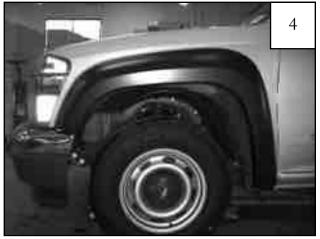
Continue until all six supplied plastic retainers have been inserted through the holes in the flare and into the holes in the fender.
