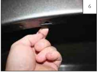
Install #10 U-Clip over existing factory holes. There are two holes at the top center location. The hole for proper installation is the one toward the front of the vehicle. *NOTE: The clip may fit over the lip loosely. This can be fixed by pinching the clip more tightly to the vehicle.*
