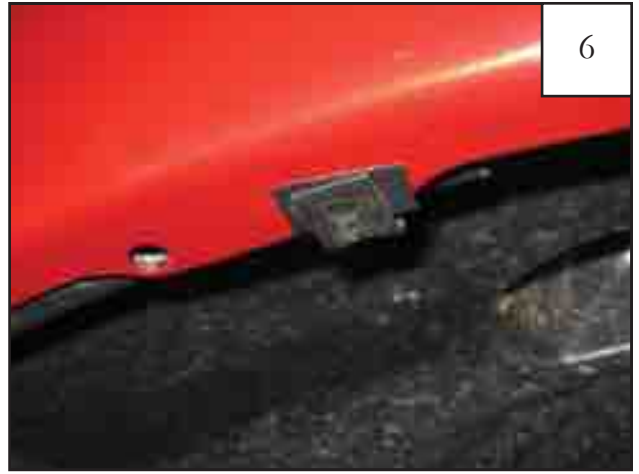
Install U-Clip over plastic tab.
