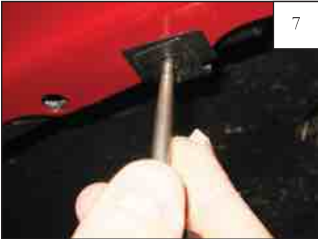
Using an awl or similar pointed tool, poke a hole through plastic tab using the speed clip hole as a guide.
