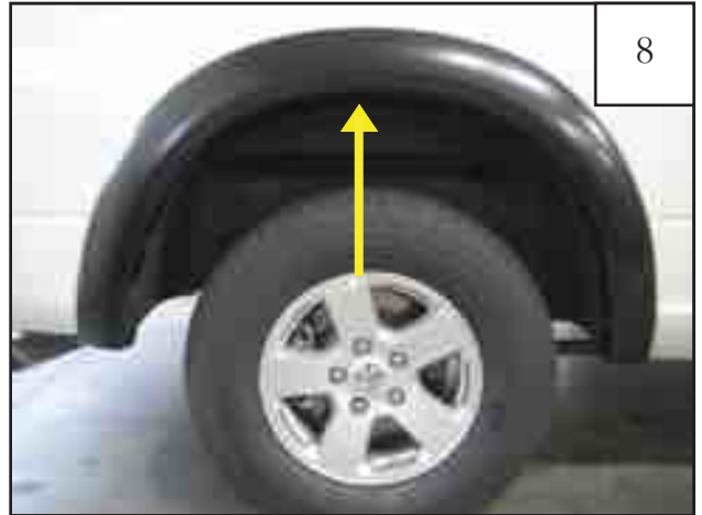
Start #8 pan-head screw using a Phillips screwdriver. Do not tighten.
