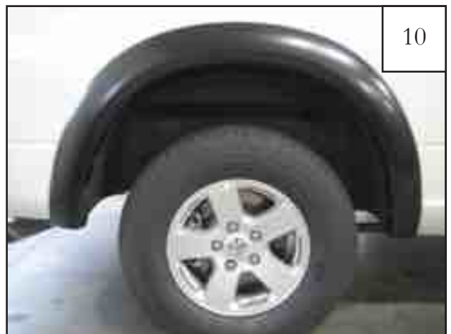
Press firmly on flare and tighten all screws. Installation Complete.
