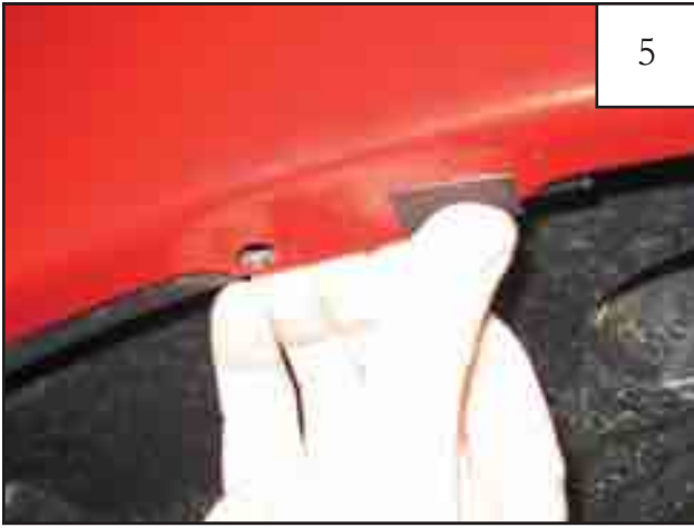
Install plastic tab over existing factory hole.
