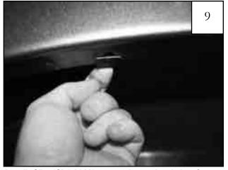
Install Clip (CL1-0022) over tabs and existing factory holes. There are two holes at the top center location. The hole for proper installation is the one toward the front of the vehicle. *NOTE: The clip may fit over the lip loosely. This can be fixed by pinching the clip more tightly to the vehicle.*
