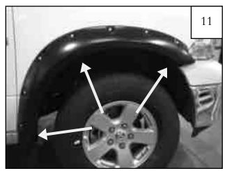
Hold flare to the vehicle and start the supplied screws with a Phillips Head Screwdriver through the factory holes. *Do not tighten.*
