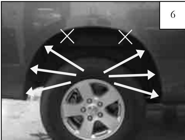
Remove these six factory installed screws using an 8mm socket wrench. X's indicate a factory screw that will not be removed.
