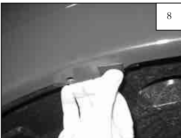
Install plastic tab over existing factory hole.
