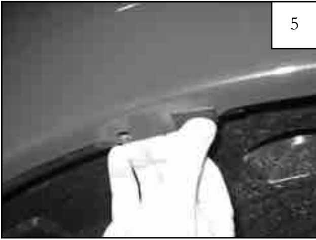
Install 1"x1.5" Black Tab over existing factory hole. There are two holes at the top center location. Refer to step 4 for proper hole for installation.
