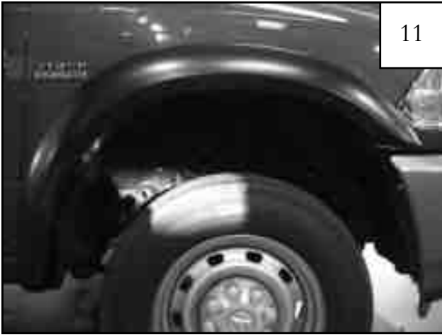
Completed front flare installation.
