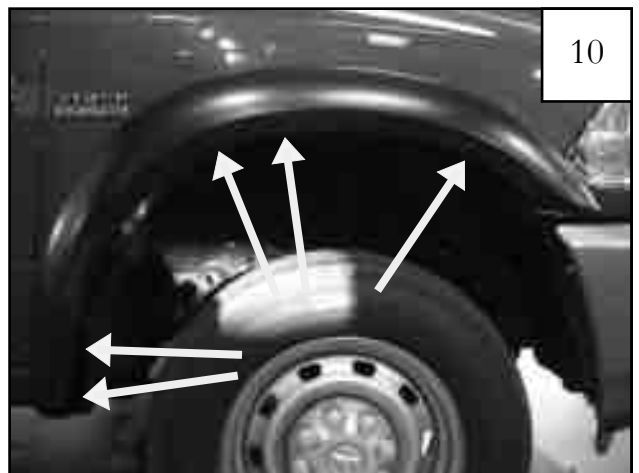
Press firmly on flare and tighten all screws.
