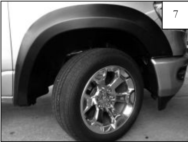
Completed front flare installation.
