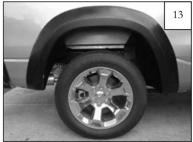
Completed rear flare installation.
