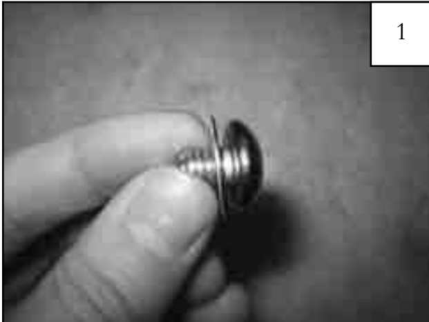
Put a Washer (WA1-0010) on each Bolt (SW1-0067).
