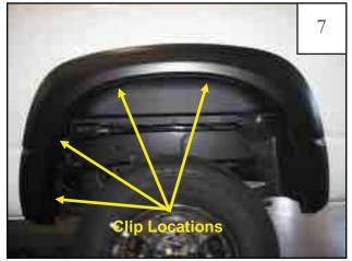
Slide a supplied clip (CL1-0009) over fender lip, aligning with existing holes (4 locations) in fender flare.
