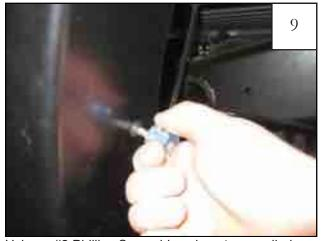
Using a #2 Phillips Screwdriver, insert a supplied Truss Head Screw (SW1-0056) through existing holes in flare and into holes of clips installed in Step 7.
