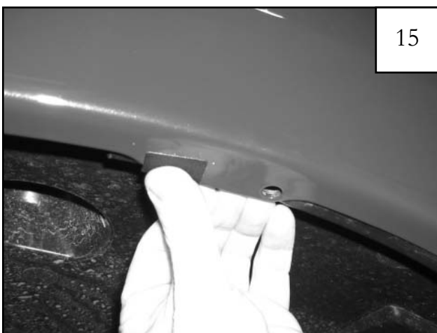
Install plastic tab over existing factory hole.
