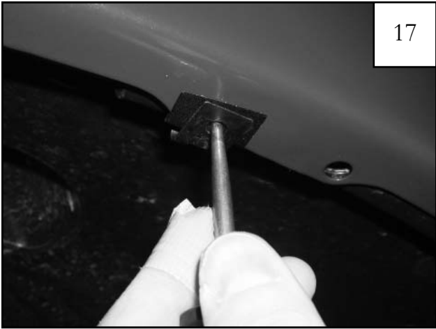
Using an awl or similar pointed tool, poke a hole through plastic tab using the U-Clip hole as a guide.
