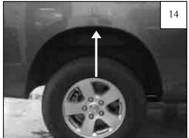
Install #10 U-Clip in this location. See steps 15 & 16.
