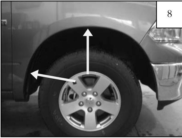
Install Clips (CL1-0022) at these locations. See Steps 9-10.
