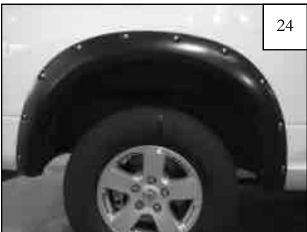
Completed rear flare installation.
