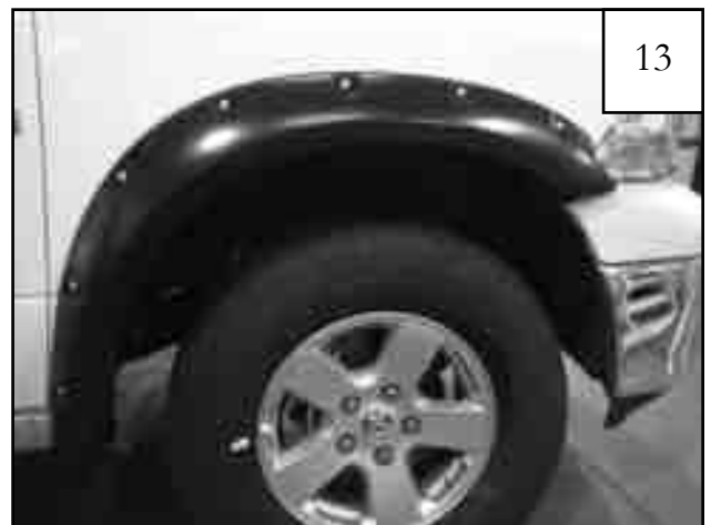
Completed front flare installation.
