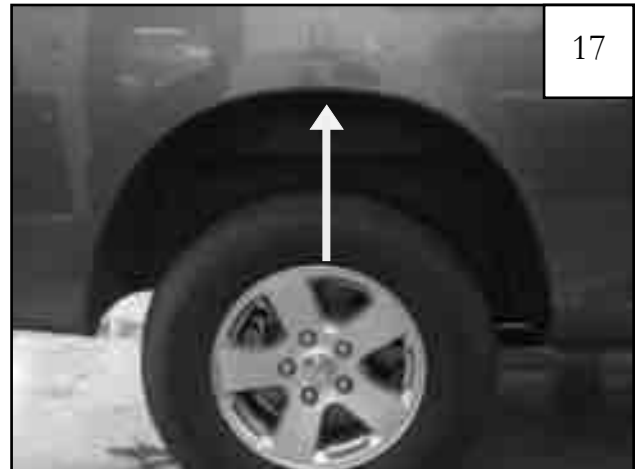
Install Clip (CL1-0022) in this location. See step 19.
