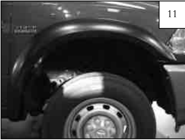
Completed front flare installation.
