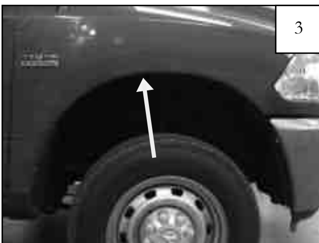
Install 1"x1.5" Black Tab and #10 U-Clip at this location. See steps 4, 5, 6, & 7.
