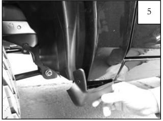
**2011-2014 Models Only:** Remove inner piece at bottom rear of wheel well.
