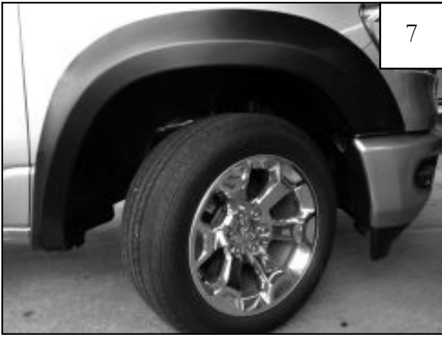
Completed front flare installation.
