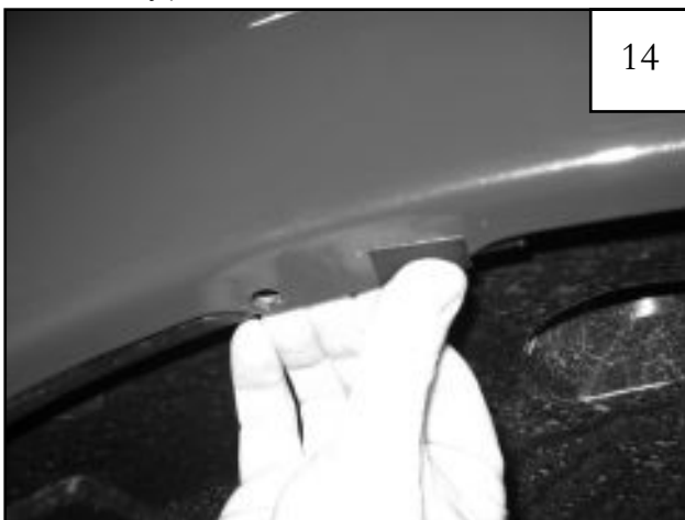
Install plastic tab over existing factory hole.
