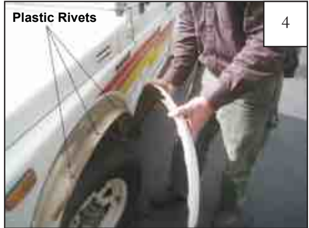
Remove all plastic rivets from the metal lip and discard.
