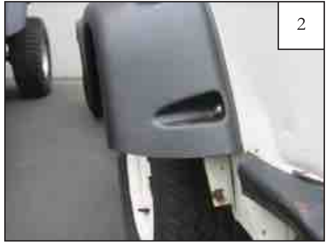
If labels have fallen off during shipping, the shorter leg of the front flare is trimmed close to the forwardmost pocket and the shorter leg of the rear flare is trimmed approximately an inch and a half from the pocket. Pictured above is the rear flare.
