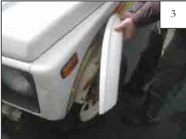
Starting at front of factory flare, pull up then out on flare to pop it off the metal lip. This will also pull the plastic rivets out of the holes in the factory flare.
