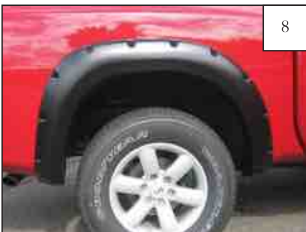
Passenger Side Flare: Completed rear flare installation.
