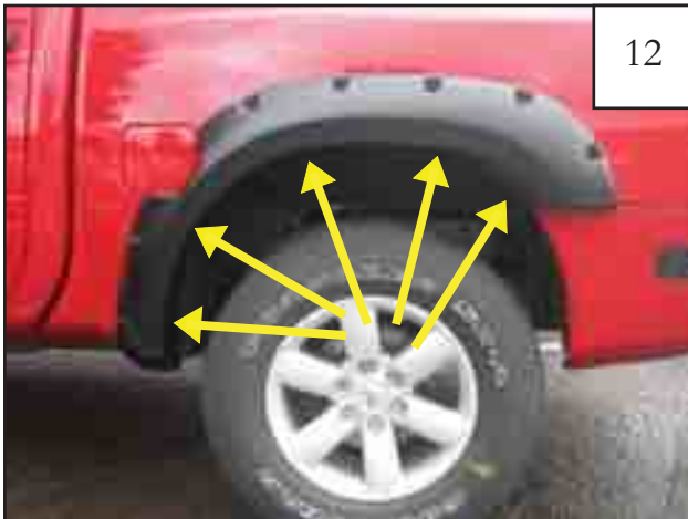
Driver Side Flare: Insuring the flare is properly located on fender, apply moderate pressure to outside surface of flare, and tighten screws, beginning with the lower front screw working toward the access door.
