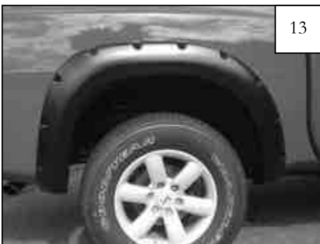
Passenger Side Flare: Completed rear flare installation.
