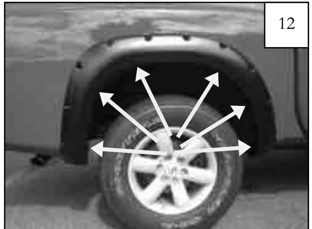
Passenger Side Flare: Insuring the flare is properly located on fender, apply moderate pressure to outside surface of flare, tighten all screws, beginning with the factory screw working toward the front of the fender flare.
