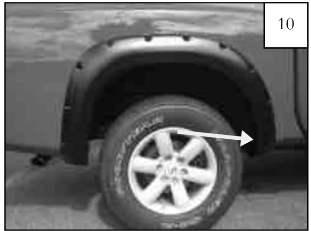
Passenger Side Flare: Hold (RR) flare in position on fender with moderate pressure. Line up the lowest hole in fender with the hole in flare and start the factory screw. Do not fully tighten screws.
