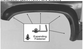
Place the flare on the vehicle. Apply 5 Plastic Expanding Fasteners into the mounting slots in the flare and secure it to the vehicle as shown.
