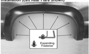
Place the flare on the vehicle. Apply 7 Plastic Expanding Fasteners into the mounting slots in the flare and secure it to the vehicle as shown.
