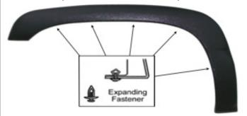
Place the flare on the vehicle. Apply 5 Plastic Expanding Fasteners into the mounting slots in the flare and secure it to the vehicle as shown.
