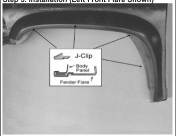
Place the flare on the vehicle. Apply 4 J-Clips into the mounting slots in the flare and secure it to the vehicle as shown.
