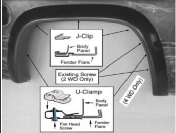
Place the flare on the vehicle. Apply 3 J-Clips into the mounting slots in the flare and secure it to the vehicle as shown. 2 U-Clamps secure into the fole with flat head scews as shows. Fasten the existing factory screws into the original location that were previously removed for 2 WD.
